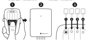
Repeat steps 1-3 to connect a new transceiver. You can connect up to 4 units.
