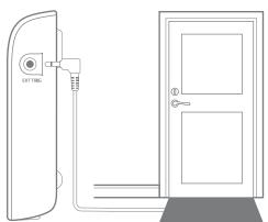
Connect the contact mat to the ext. trig. outlet on the Visit telephone transmitter.
