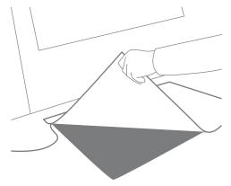
Place the contact mat on a flat, smooth surface and mount the cables to the wall or baseboard.
