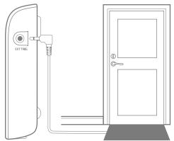
**2.** Connect the Contact Mat to the ext. trig. outlet on the Visit transmitter.
