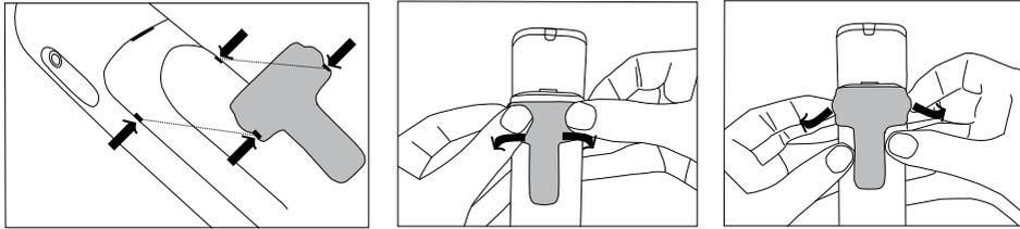
Place the clip against the battery cover and press firmly so that it locks on.
